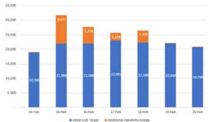
WAPA worked with the U.S. Army Corps of Engineers Feb. 15 to 18 to increase generation from the Missouri River power plants to support the grid. This graph shows the additional hydropower that the Corps provided during Winter Storm Uri.
